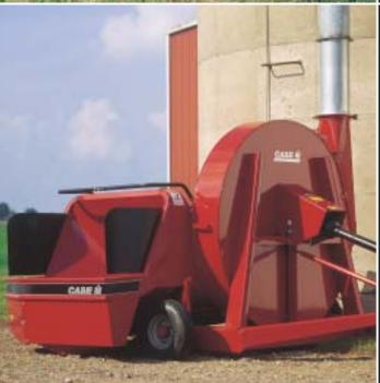
For a forage blower that can keep up with the FHX300 and your wagons and trucks, choose the Case IH 600 forage blower. It fills extra-tall silos fast to increase your productivity. Features include an auger-fed design and a 60-in. (1524 mm) diameter blower fan.
