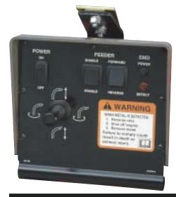
A light and horn alert you when metal is detected. Just use the feedroll control switch to back the material out of the feedrolls. After the metal has been removed, the metal detector resets automatically.
