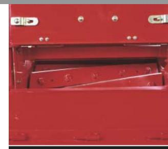
At the heart of the Case IH Model FHX300 is this 21-in.-diameter, 12-knife cutterhead. Hardened alloy knives span the full width of the cutterhead and chop evenly and efficiently, converting your crop into high-quality feed.
