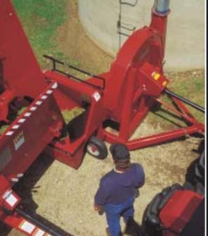
You can position wagons fast thanks to the wide 37-in. (940 mm) hopper that extends 20 in. (508 mm) past the blower housing. You'll have ample room for maneuvering into position and easy access to speed up your unloading time.
