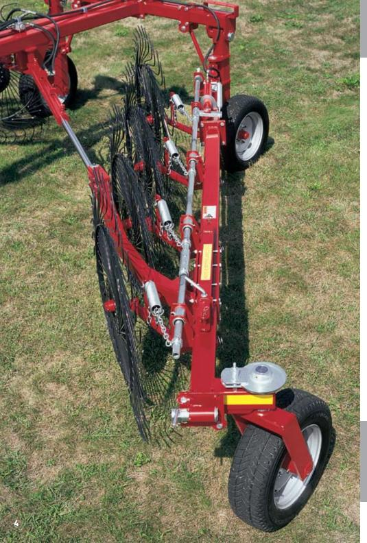
Swing cylinders quickly and easily expand raking wheels from transport to working position.
