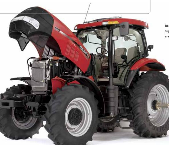
Rear-pivot front-release hood is supported by gas-filled cylinders, making it easy to raise.
