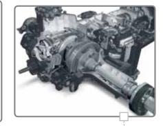
Full Powershift transmission, .....: provides seamless smooth shifting from zero to 40 or 50 kph. Optional CVT transmission for improved fuel consumption and operator comfort. Creeper gears offer an additional 10 speeds from 225m/h to 1.6 kph @ 2,200 rpm.
